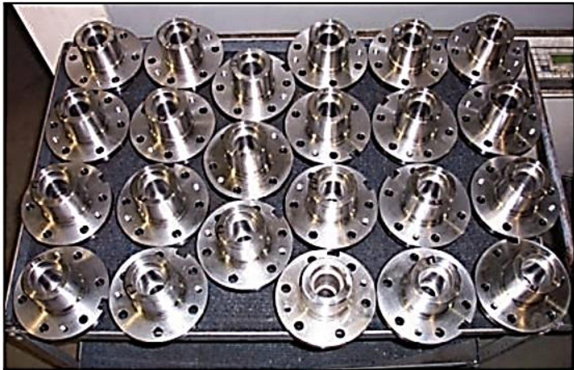
Wire EDMing Internal Keyways
